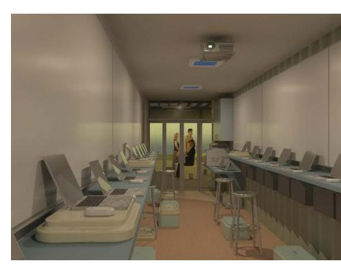
The entry storefront is designed to minimize heat gain / loss by use of a less-than-standard size door: 1'-7" x 6'-4" (48 x 193cm). Wheelchair access is made possible by opening the normally fixed panel to provide 38" (~1m) of clear area. In front of the storefront glazing is a second strip door made of clear plastic strips that allow you to pass through but inhibits air movement creating a mini airlock.
