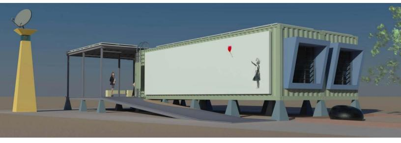
The design contains two ancillary elements. The tower will function as the security guard's station and generator garage but also to mark location. At night a beacon will illuminate the grounds as a security measure. The fixture will have a light cut-off to avoid trespass beyond the immediate area. Additionally, there will be area lighting for 24 hour operation of the lab.
